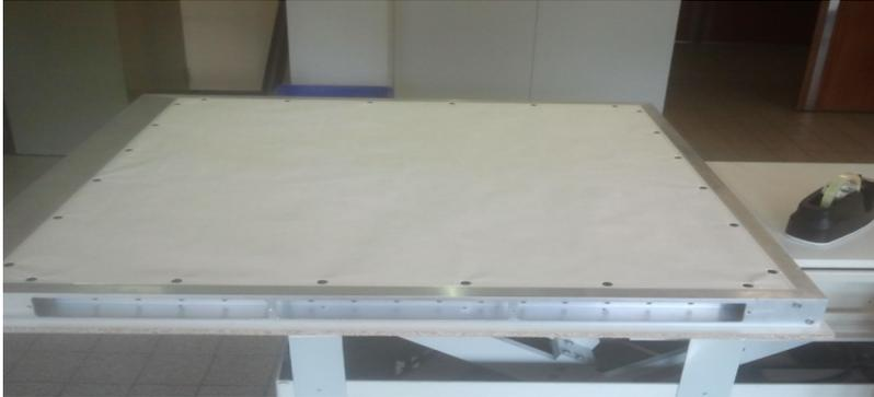
**Figure 5.11:** Picture showing the back of an aluminium frame equipped with a big Tyvek sheet.
