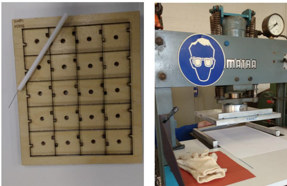
**Figure 5.6:** Pictures of the wooden tool (left) and the press (right) used to cut the punched Li screens.
