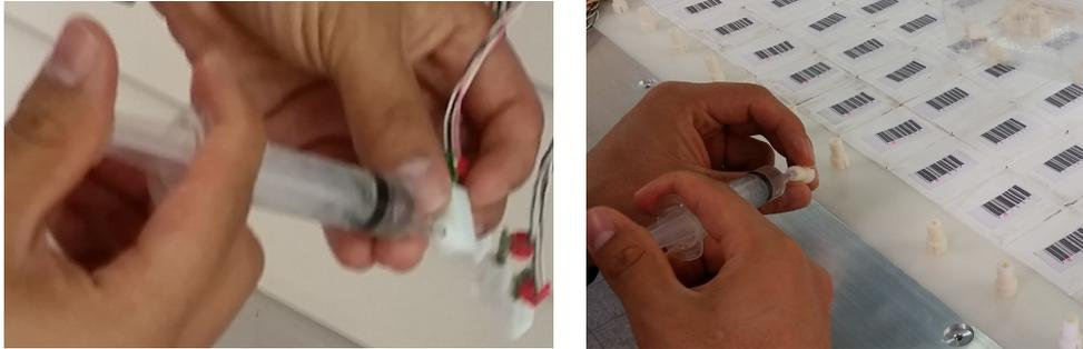
**Figure 5.17:** Application of optical grease with the help of a syringe for the MPPC connector (left) and the mirror connector (right).
