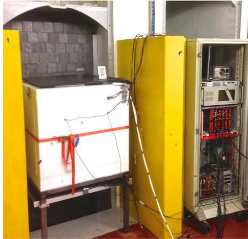
**Figure 2.6:** NEMENIX inside HDPE shielding placed in front of the BR2 reactor. 2 muon detectors wrapped in black plastic are visible below and on top of the shielding.
