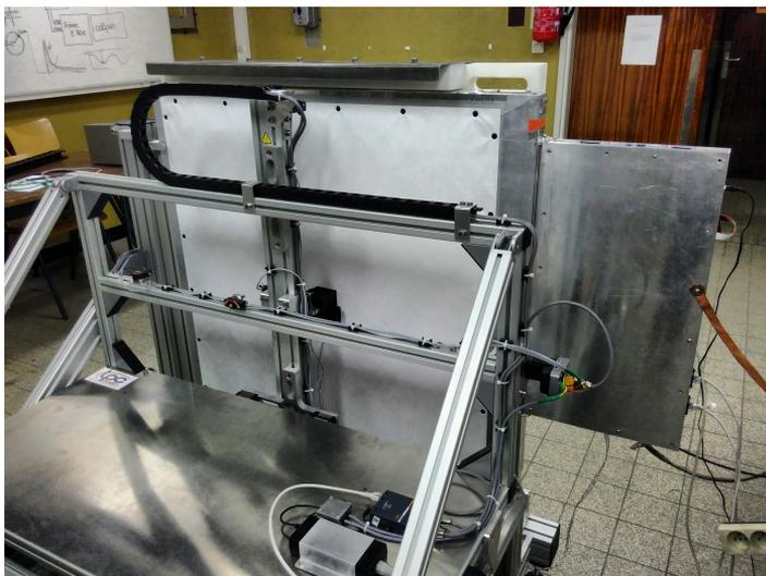
**Figure 5.19:** Calipso set-up for the EM source measurements. The black box positioned at the middle of the frame holds the EM source.
