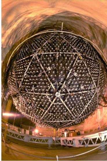
**Figure 1.6:** The Sudbury Neutrino Observatory 12m diameter vessel [37].
