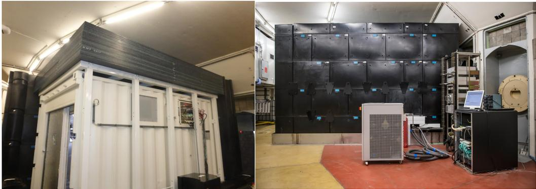
**Figure 5.3:** The left figure shows the HDPE plates on top of the container. The right figure shows the closed water wall from the side. The cooling system and the electronics rack are also visible.
