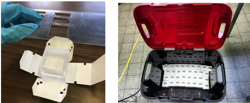
**Figure 5.9:** Pictures showing the metal template used to position the cube correctly within the Tyvek (left) and the cube storage box (right).
