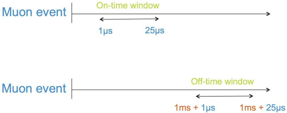
**Figure 6.23:** Schematic representation of the on-time and off-time window approach used for the study of Michel electrons.
