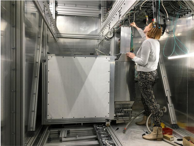
**Figure 5.2:** Picture of 1 module inserted in the container. Electronics boxes, fans and service box are visible.
