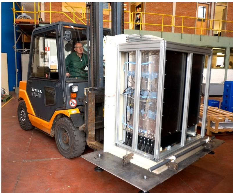
**Figure 3.4:** The SM1 prototype with the bottom and back side of the shielding and the steel plate attached.
