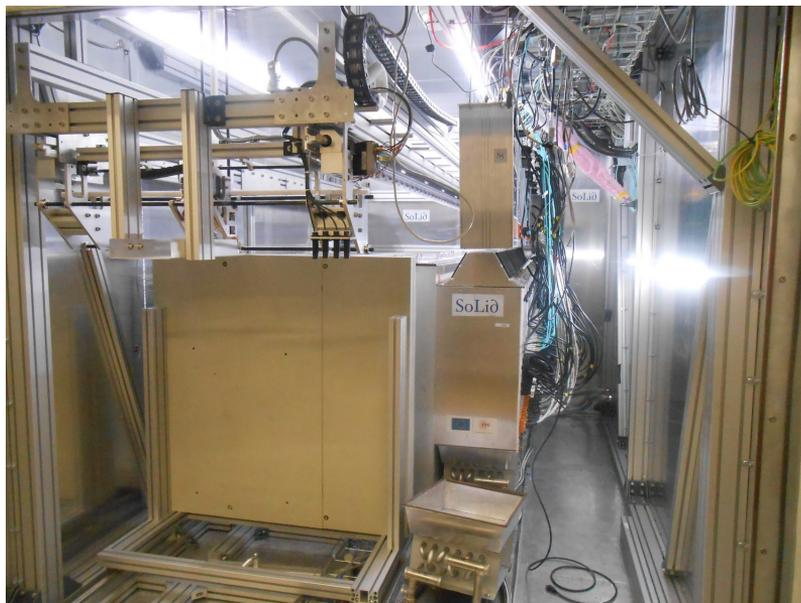
**Figure 5.4:** Picture of 4 modules inserted in the container, plus 2 HDPE plates, one at the front and 1 at the back of the container. All electronics boxes and service boxes are cabled and the cooling system is attached. In the bottom right, part of the cooling system that is foreseen for module 5 is already available. In this picture the reactor is situated at the back, behind the container.
