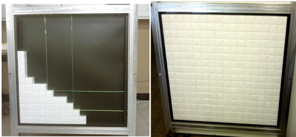
**Figure 3.5:** SM1 frame partly filled with 4 fibres inserted with black HDPE backing visible (left), filled SM1 frame with black HDPE side bars clearly visible (right).
