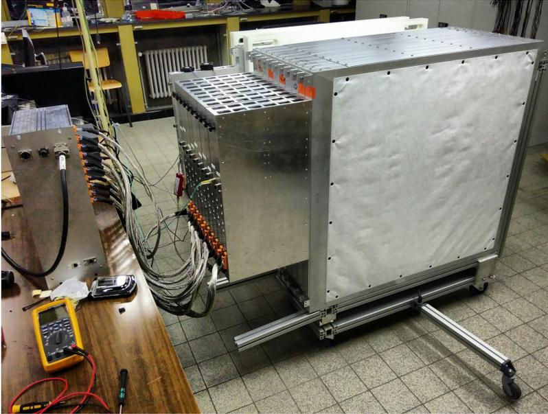
**Figure 5.1:** Picture of a Phase 1 module with electronics boxes attached in a test set-up at the Ghent University lab.
