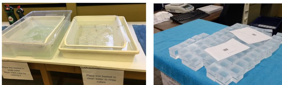
**Figure 5.7:** Pictures showing the washing, rinsing (left) and drying (right) of cubes.
