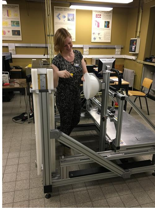
**Figure 5.20:** Calipso set-up for the neutron source measurements. The white HDPE moderating plates are visible around the frame. I am adjusting the collimator holding the  $^{252}\text{Cf}$  source.
